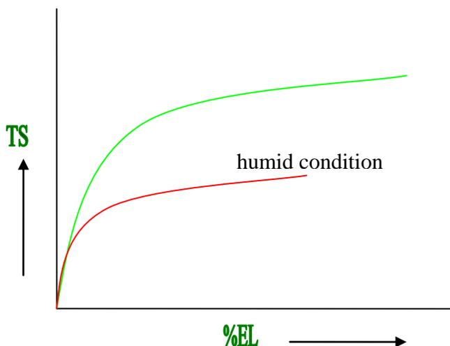
Fig. 1 Effect of moisture on mechanical properties of propellant
